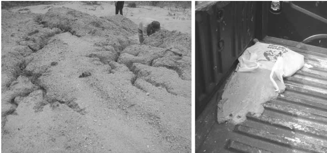
Fig. 13: Tierra Blanca Joven (TBJ) problems, on the left erosion problems; and in the right liquefaction of TBJ after vibrations in the back of pick up vehicle.
