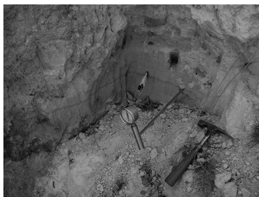
Fig. 14: Measurement of moisture content in TBJ slope (TMS1, left side of photo) and suction (tensiometer, right side of photo).
